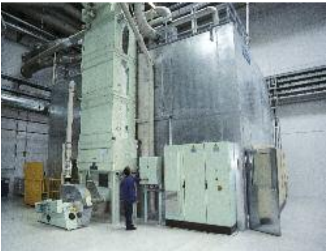
In 2000, HARTMANN set up a separation plant for production wastage in the manufacture of incontinence products at its facilities in Herbrechtingen, Germany.
